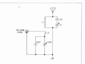
fig. 4. Coupler provides match between high impedance seen at antenna terminals and 50-ohm coax line.
